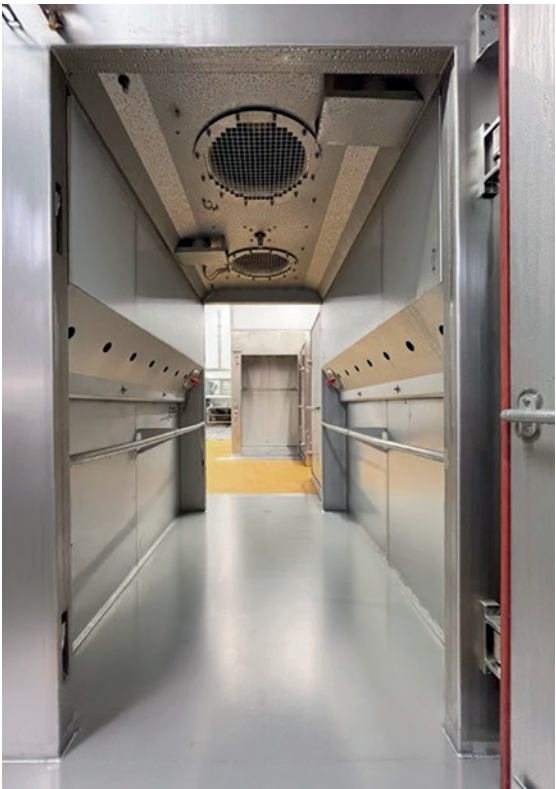
INSIDE THE INTENSIVE CHILLING SYSTEM ARCTICjet® IK-2 transit model with two variable-speed recirculation fans
