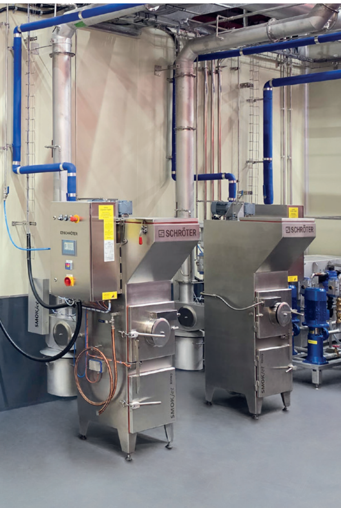
WOODCHIP SMOKE GENERATOR SMOKjet® RH09 with 1-fold exit supplies smoke to the SEMIjet®.
