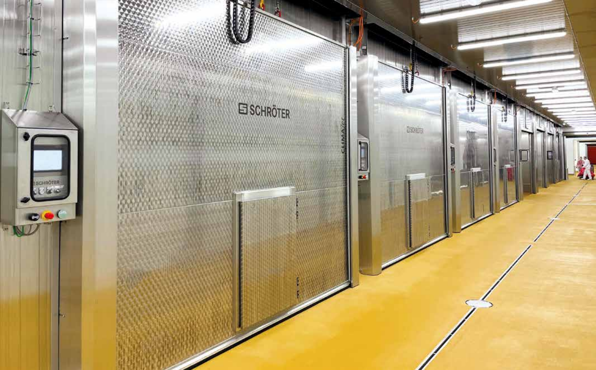
FRONT PANELS WITH LIFTING DOORS across the entire width of the system
